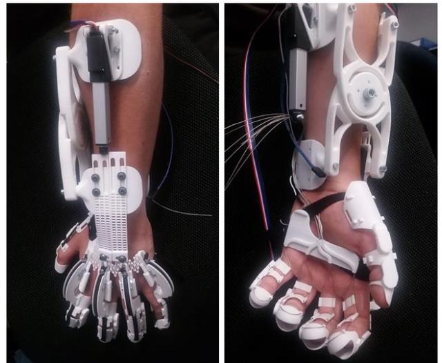
Figure: Patient using a prototype of the lightweight hand exoskeleton [University of Stuttgart].
