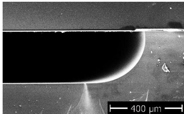
Figure 5: SEM picture of a cross-sectional view (fracture edge) of a glass substrate bonded to a structured glass substrate.
