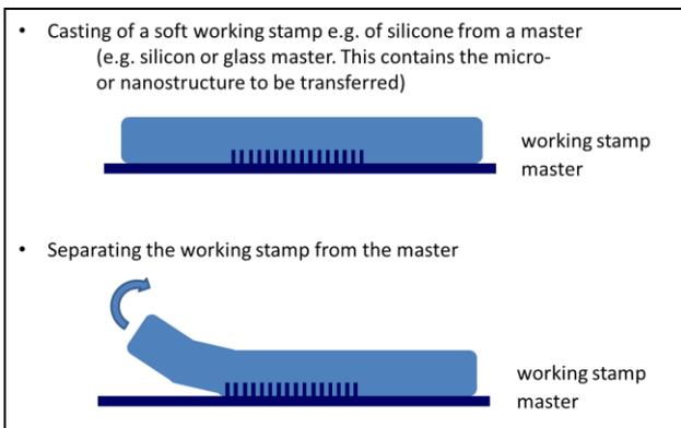
Figure 2: Microstructured lamination: Step 1 - Production of the working stamp.
