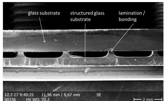
Figure 1: SEM picture of a cross-sectional view (abort edge) of a glass substrate bonded to a structured glass substrate [Image: Karlsruhe University of Applied Sciences].
