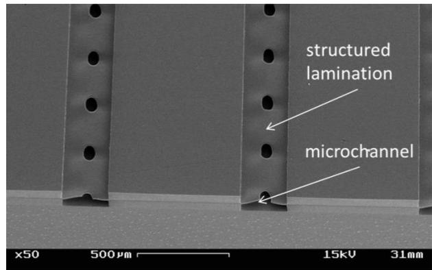
Figure 6: An additional layer may be laminated in order to obtain two channels on top of each other, so that the microfluidic component can be used e.g. as a mixer or filter.
