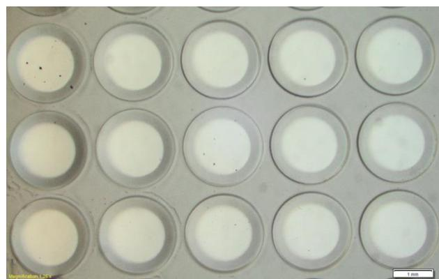
Figure 7: Light micrograph of laminated (covered) microwells in a glass substrate (scale bar 1 mm) [Images: Karlsruhe University of Applied Sciences].
