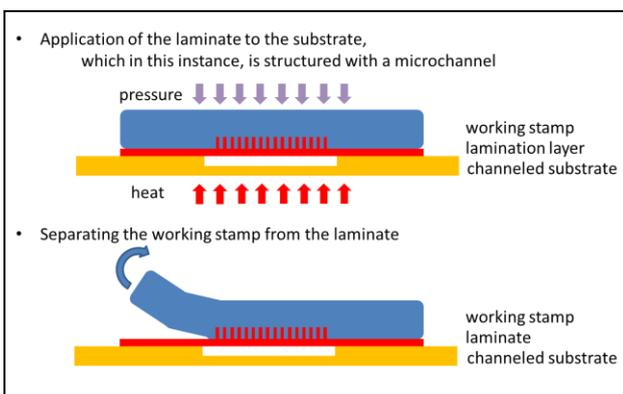
Figure 4: Microstructured lamination: Step 3 - Application of the laminate.
