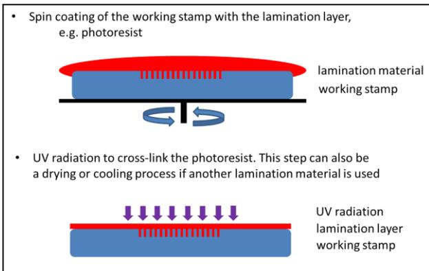
Figure 3: Microstructured lamination: Step 2 - Production of the lamination layer.
