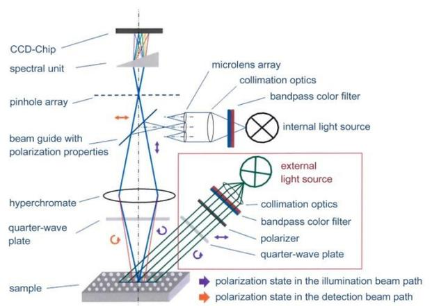
Figure: Invented design with polarized illumination and detection (with additional gloss suppression). Bandpass filters in front of both light sources are used to adjust the spectral ranges [University of Ulm].
