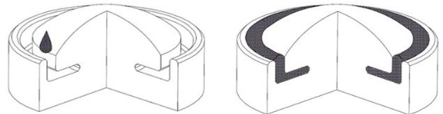
Figure: Schematic drawing of a lens with microcavity when filled with a functional substance (left); lens with resulting aperture (right).
