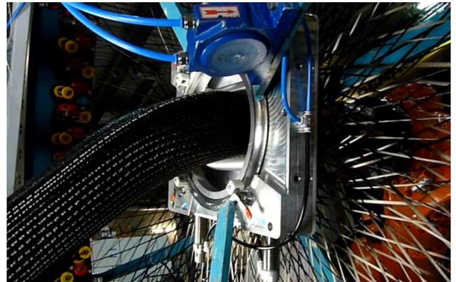
Figure 1: Pressure roll mechanism integrated into a radial braiding machine
