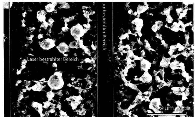
Figure1: SEM image of a silicon layer with a non-irradiated (right) and a laser-irradiated area (left).
