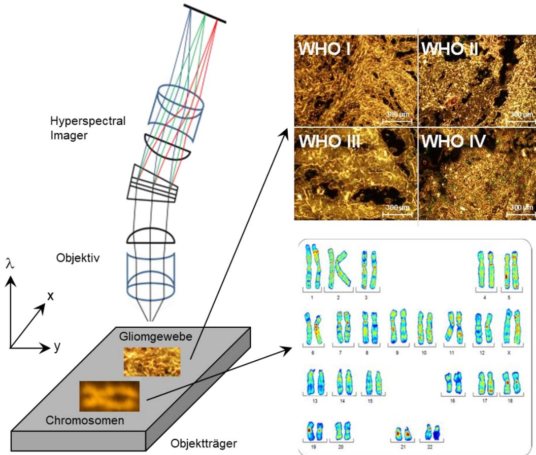
Figure 2: Using the compact spectrometry module with different software packages allows you to perform various marker-free analyses. The characterization of glioma tissue (top right) and the creation of a karyogram (bottom right) are just two examples of applications which have been successfully tested at the Institute.
