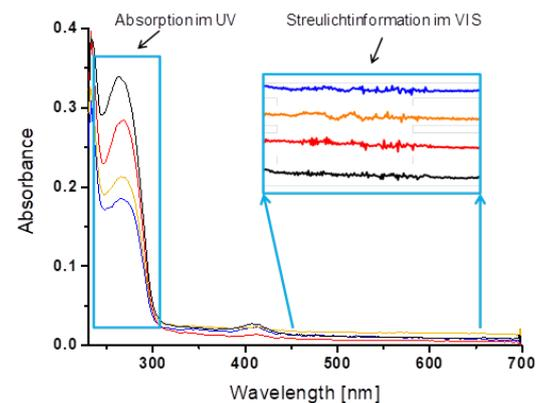
Figure 1: UV/VIS spectra with absorbance in the ultraviolet range (chemical information) and overlaid fine structures in the visible range due to scattered light interferences (morphological information).
