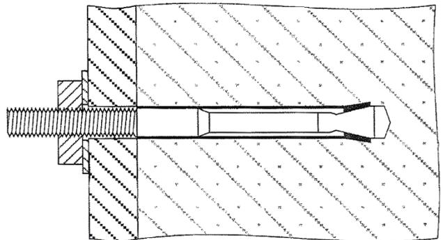
Figure: Schematic drawing of the ductile seismic anchor.
