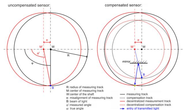
Figure 1: Encoder reading without compensation (left) and with compensation track (image: ITO, University of Stuttgart)
