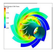
The basic idea of the MEDUSA control concept is to divide the turbine inlet into several sectors along the circumference and to control the inflow of the various sectors individually by means of valves. (Graphic: University of Stuttgart)
