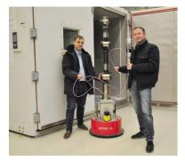
Prof. Dr.-Ing. Bernd Langer (right) and Prof. Dr.-Ing. Martin Kipfmüller at the Karlsruhe University of Applied Sciences have developed a process for the automated production and assembly of cable harnesses. By cooling the cables, a flexurally rigid state is achieved, so that industrial robots can be used flexibly and economically for the production of cable harnesses. Foto: TLB GmbH
