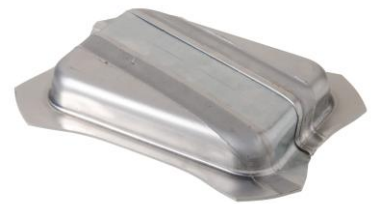
Exemplary technology demonstrators of formed, hybrid TWBs made of aluminum and steel. (Photos: Stuttgart University)
