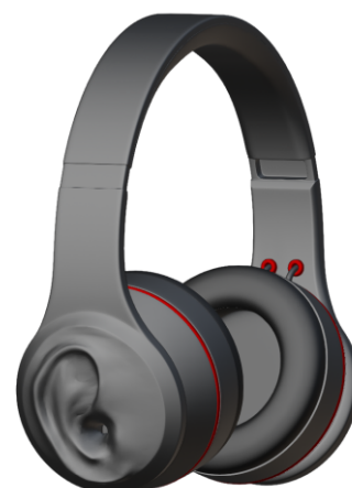
Sketch of a possible headphone prototype with the innovative filter element. In this example, the shaped structures (protrusions) share the natural shape of the human ear, but other designs are also possible. [Fig.: Timo Oess]
