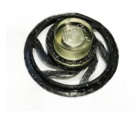
The spring element for the Exciter is made of endless fibre-reinforced plastics that are thermally conductive. Photos: Benjamin Grisin
