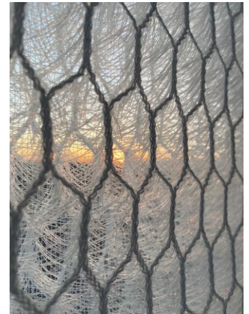
The core element of HydroSKIN is a so-called spacer fabric, two textile layers, which are kept apart by threads and thus well-ventilated.
