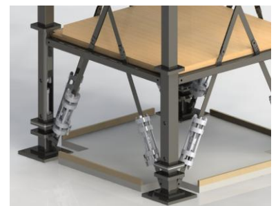
Researchers at the University of Stuttgart have developed active, adaptive structural elements that can be used to manipulate the load transfer behaviour in a structure. (Photo: ISYS + IKTD, University of Stuttgart)
